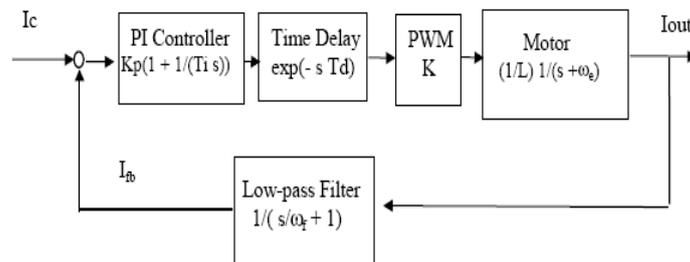
Fig. 3(b) Block Diagram of a Current-loop
