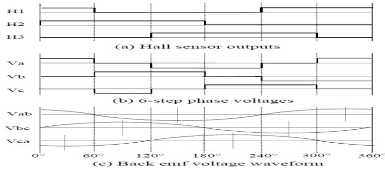
Fig. 2. 120° Conduction Commutation
