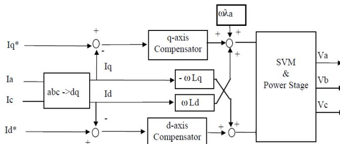
Fig. 3(a). Synchronous Regulator with Decoupling Control
