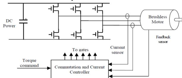
Fig. 1. Block Diagram of a Brushless Motor Drive System
